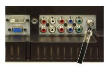
Coaxial (RF) carries the video and audio from one cable. The coaxial connector is labeled, ANT/Cable on your TV display. To locate the connector, see page 8.
